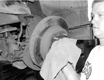
5. Remove the nut securing the tie rod end to the spindle. Use a ball joint puller to separate the tie rod end from the spindle. Remove the dust cap from the rotor, remove the cotter pin and castle nut from the axle and slide the rotor off the spindle. Keep the wheel bearings inside the rotor and set everything aside.
