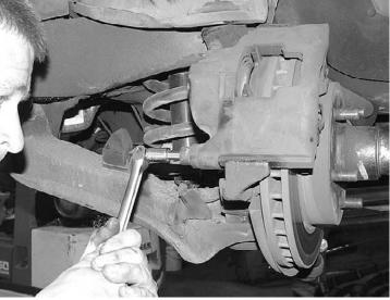
4. Position the brake line as shown above and tighten the 2 bolts. Lubricate the brake line with some light oil and pull the extra slack down toward the brake caliper. Remove the 2 bolts securing the brake caliper to the spindle, slide the caliper off the spindle and tie it up against the frame rail. **DO NOT LET THE CALIPER HANG FROM THE BRAKE LINE!**
