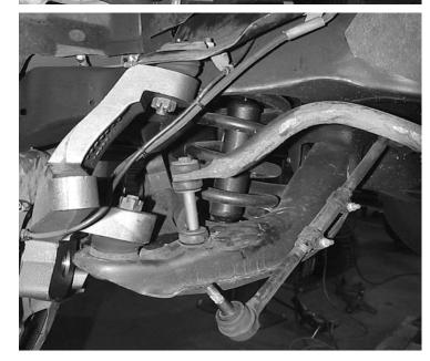
12. Slide the ABS sensor wire behind the steering arm. Route the wire along the rubber brake line and place it back in the retaining clip on the upper ball joint. Using the supplied cable ties, attach the wire to the brake line. Tighten the retaining clip on the upper ball joint, do not crimp the wire.
