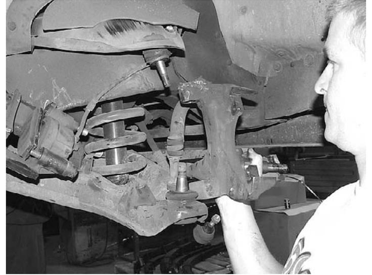
6. Remove the three bolts securing the dust shield to the spindle and set the shield aside. Remove the rubber ring from the spindle and set this aside with the dust shield, they will be reinstalled later.
