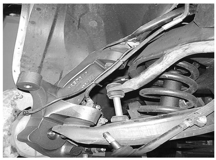
11. Separate the ABS sensor wire from the retaining clip on the upper ball joint. Slide the rubber ring onto the lift spindle, followed by the dust cover and ABS sensor. Reinstall the three original bolts.
