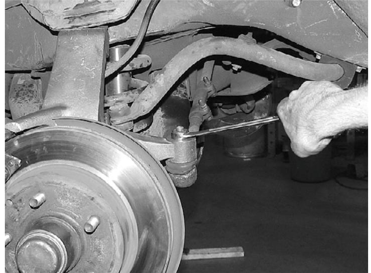
15. Attach the tie rod end to the spindle and retorque the original nut to factory specs.
