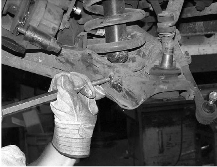
8. Grind the heads off the rivets securing the steering stop to the backside of the LCA. Using a punch or air chisel, remove the rivets and steering stop from the LCA.
