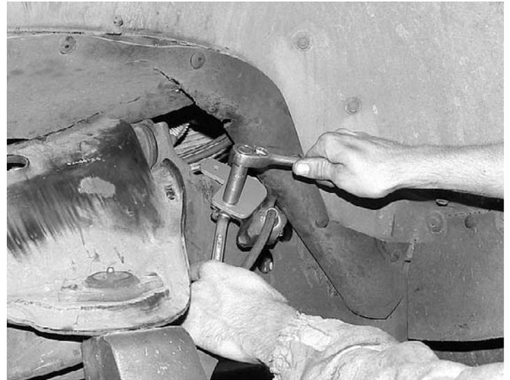
3. Attach the brake line relocation tab to the top of the frame rail using the original bolt, only hand tighten. Using the supplied 1/4" bolt, flat washers and lock nut, attach the brake line to the relocating tab. You may have to slightly bend the factory hard line. **MAKE ONLY SLIGHT BENDS, DO NOT KINK THE BRAKE LINE.**
