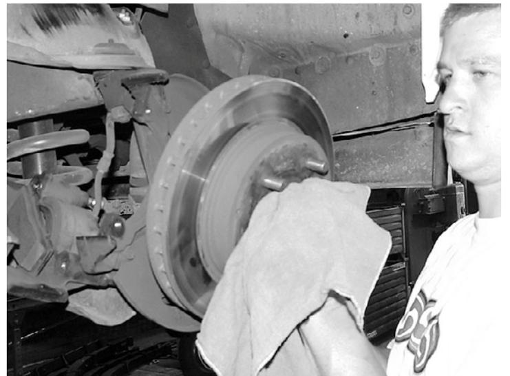
5. Remove the nut securing the tie rod end to the spindle. Use a ball joint puller to separate the tie rod end from the spindle. Remove the dust cap from the rotor, remove the cotter pin and castle nut from the axle and slide the rotor off the spindle. Keep the wheel bearings inside the rotor and set everything aside.
