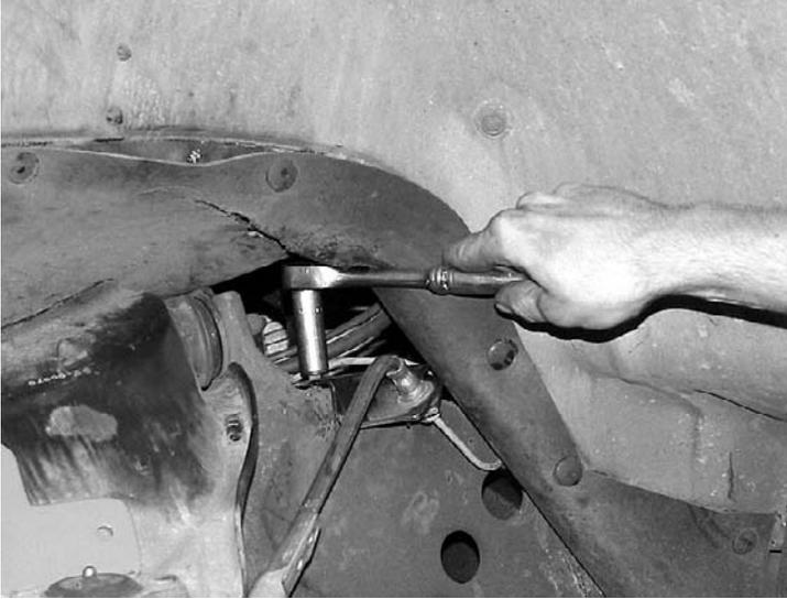
2. Starting on the passenger's side, remove the front tire. Remove the 2 bolts securing the brake line tab to the upper control arm (UCA). Remove the bolt securing the brake line mount to the top of the frame rail.
