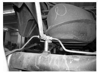
3. Locate the Portioning Valve on the passenger side of the axle. Remove the valve from the axle and save the hardware. Locate FT70033 proportioning valve ext. and attach to the axle use the factory hardware. Attach the proportioning valve to the new bracket using the supplied 5/16" bolt, nut, and washers. SEE PHOTO BELOW.
