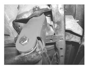
6. Locate the factory lower rear bumper bolts. Remove and discard the bolts. Locate the supplied 10mm x 20mm bolt and washer and install were the previous bumper bolt was removed. Use a small amount of the supplied thread lock compound on the bumper bolts before installing.
