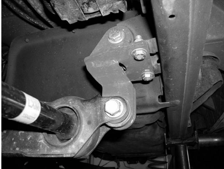
5. Install the factory torsion bar crossmember to the new bracket using the stock hardware. Torque both of the bushing eye bolts to 50ft-lbs.
