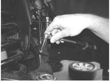
3. Loosen the upper ball joint nut, strike the knuckle with a hammer till it comes loose from A-Arm. Save all hardware. (Use care not to hit threads.) SEE PHOTO IN NEXT COLUMN.
