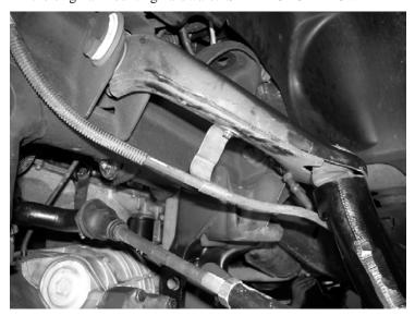
38. Reinstall the torsion bars by pulling them through the torsion bar relocater bracket and then sliding it back into the factory torsion key. Set the torsion adjuster to the premeasured height. SEE PHOTO BELOW.
