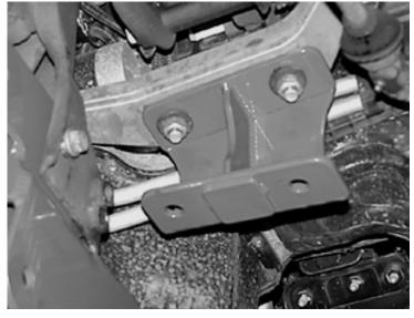
25. Place the differential housing into the Fabtech rear crossmember using the stock hardware on the driver side and 9/16"-12 x 1-3/4" bolts, nuts and washers on the passenger side from hardware kit FT20465, leave loose. SEE PHOTO BELOW
