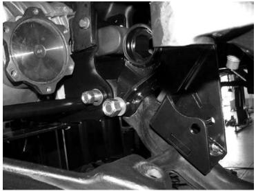
34. Locate the FT20246D & P steering knuckle and install the stock hub bearing assembly taking care to place O ring in the proper position. Apply thread lock compound to the stock hardware torque the flange bolts to 130 ft-lbs. SEE PHOTO BELOW.
