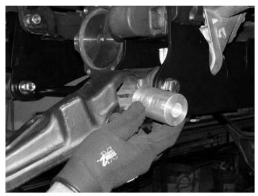
33. Locate the Torsion Bar Relocator FT20455BK and install it on to the lower control arm using the factory shock mount bolts and the supplied ¾"-10 x 4-1/2" hardware. Torque the factory bolts to 58 ft-lbs and the ¾ to 450 ft-lbs. SEE PHOTOS BELOW
