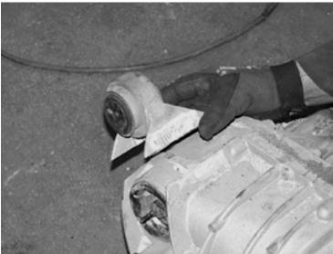
19. On some model trucks, the differential has a small area the needs to be sanded down level to allow the supplied Drv. Diff bracket to fit flush against the diff. Using a sanding disc, sand the differential as shown in the following two pictures. USE CARE TO NOT SAND TOO FAR, YOU WILL ONLY NEED TO APPROX. 1/4". SEE PHOTO BELOW.
