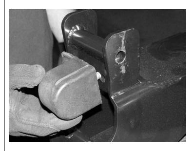
23. Install the Rear crossmember into the rear lower control arm pockets on the vehicle. SEE PHOTO BELOW.
