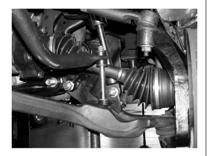
43. Recheck all bolts on front end for proper torque before proceeding to next step.
