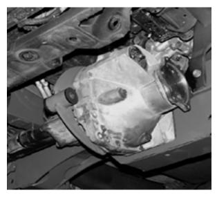
26. Position the front differential urethane bushing mount into the front crossmember tabs. Locate and install the differential skid plate around the differential housing bushing using 9/16"x 5" bolt, nut and washers from hardware kit FT20076. Leave loose.
