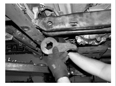
39. Install Fabtech shock part number FTS7191 (not included) using  $9/16 - 12 \times 4 - 1/2$  hardware. Torque the upper stem bushing to 15 f t-lbs and the lower bolt to 129 ft-lbs.
