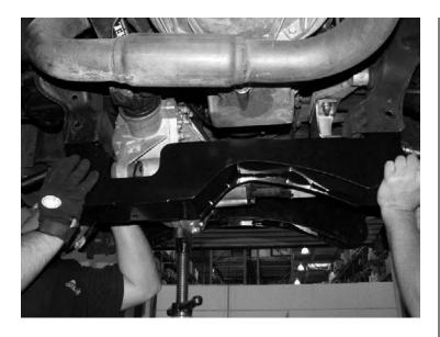
24. Locate and install the Fabtech Passenger side Diff bracket FT20061 to the bottom of the factory frame mount, with the wide end of the bracket to front of the vehicle. Attach using the stock hardware. Torque to 70 ft-lbs. SEE PHOTO BELOW.
