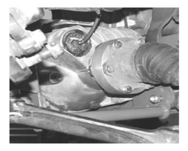
37. Locate the factory brake line mount on top of the upper control arm. Remove the brake line mount and route the line with bracket to the bottom side of the control arm. Drill a 13/64" hole directly below the original hole on the upper control arm. Mount the factory bracket to the bottom side of the control arm using the original mounting hardware. SEE PHOTO BELOW
