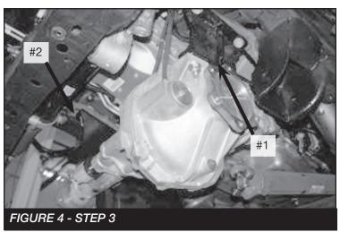
4. Install the new rear diff support bracket (Part #3) Leave loose. **SEE FIGURE 4**
