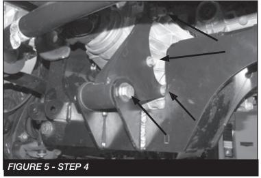
5. Torque all of the differential hardware to spec. Install the new CV driveshaft. Reinstall the skid plate with the hardware removed in step 1. Torque ½" skid plate hardware to 75 ft-lbs., and the 7/16" to 50 ft-lbs.
