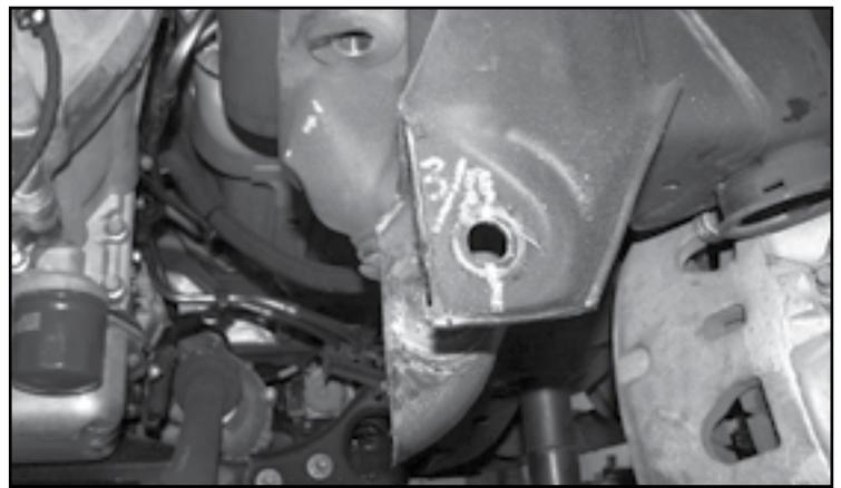
18. Locate the passenger side lower control arm pocket. From the center or the control arm pivot hole, measure  $1-3/8$ " down and make a straight line across on the front side only. Using a sawzall, cut the front portion of the pocket only. **SEE FIGURES 14-15**
