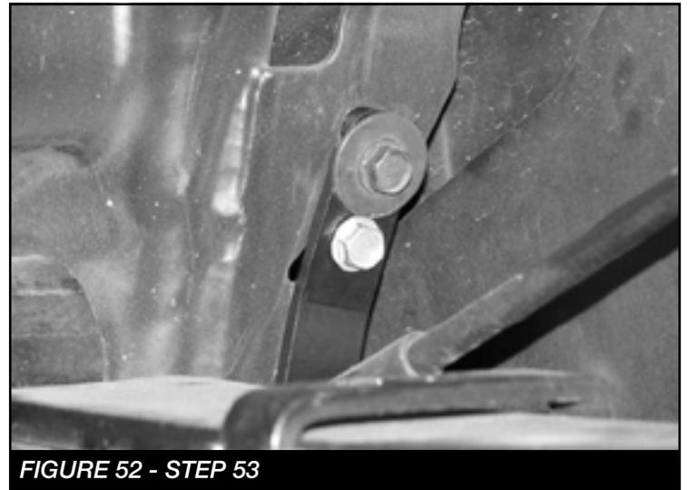
54. Install the new Fabtech shocks with the factory hardware. On Performance and Stealth shocks use one 9/16" washer per side on both upper and lower mounts torque to 100 ft-lbs.
