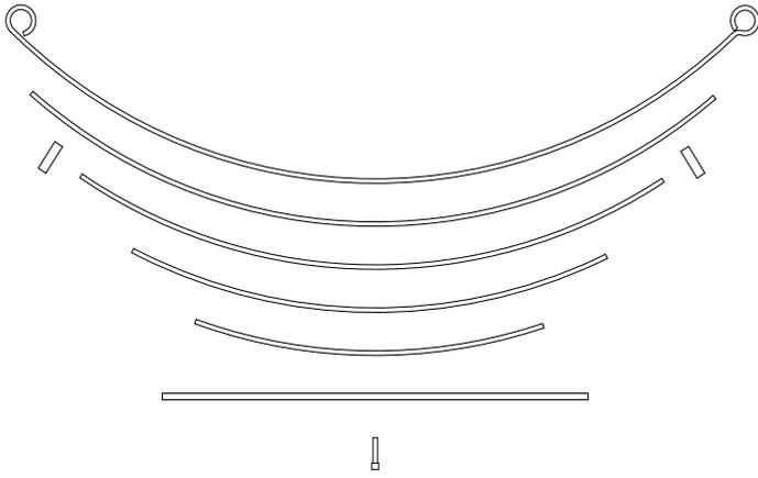
4. Realign the center pin in the leaf spring pack to the centering hole on the axle perch and install the original u-bolts. Torque u-bolts to manufacture specifications.
