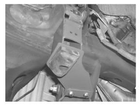
18. Locate the previously remove brake line tab from the frame. You will need to carefully pull the hard line 4" down the frame to the new mounting bracket. Using the supplied ¼" bolt, nut, and washer attach the brake line tab to the Fabtech bump stop mount. SEE PHOTO BELOW
