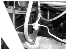
38. Locate the factory E-Brake Cable on the driver side rear hub and remove the e-brake cable from the hub bracket. Locate the supplied FT30043 E-brake cable extension, using the supplied ½"x 1 ½" bolt, nut and washer, attach to the factory bracket on the hub. Attach the E-Brake cable to the new bracket the same way it was attached to the factory hub. SEE PHOTO BELOW.
