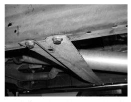
37. Locate the factory brake line mount on the driver side of the axel. Remove the vent line from the bolt and remove bolt, save hardware. Locate the supplied brake line bracket FT30042, attach the side with the sleeve to the axel using the factory hardware. Using the supplied 3/8" x 1 3/4" bolt, nut, and washer attach the brake line to the other end. Reattach vent line. SEE PHOTO BELOW.
