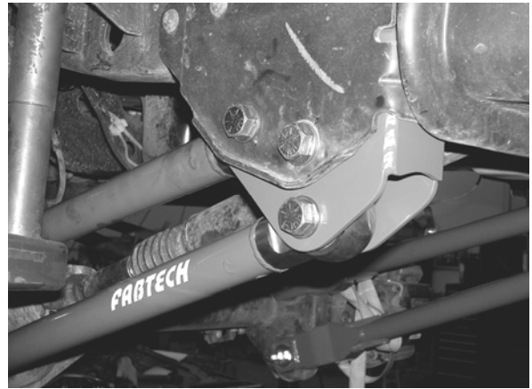
Assembly of the FT292 Alignment Cam
