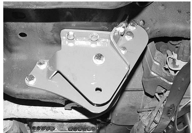
Driver Side I-beam Bracket Passenger I-Beam connection point
