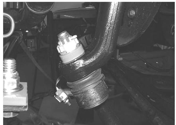
26. Locate the supplied FT30205 stabilizer bracket and install it in the factory location using the original hardware and torque to 65 ft. lbs. Re-connect the stabilizer to the new drop bracket and tighten to 45lbs. SEE PHOTO BELOW.
