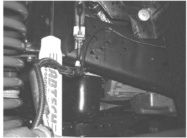
24. Locate FT30169BK sway bar frame drop bracket and attach it to the frame using the original sway bar hardware. Attach the sway bar to the new frame mounts using the supplied 7/16-14 x 1 1/2" bolts, nuts and washers. Attach the end links to the stock spring perch's on the I-Beams using the original hardware. Torque the end link hardware to 55 ft. lbs and the frame mount hardware to 45 ft. lbs. SEE PHOTO BELOW.
