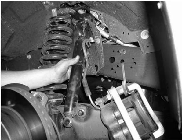
3. Working from the driver side of the truck, support the I-beam with a jack and remove the J clip at the top of the coil spring. **EXERCISE EXTREME CAUTION WHEN WORKING WITH COIL SPRINGS UNDER LOAD!** Lower the floor jack supporting the I-beam and remove the nut at the bottom of the coil spring. Discard the coil spring, and save all hardware.
