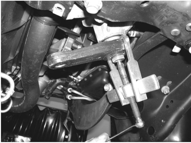
11. Locate FTS30122 new drop pitman arm. Attach to the steering box in the same indexed position as the factory pitman arm was when removed. **Install the provided FT30258 Sector Shaft Nut and torque to 350 ft. lbs. (Note: this is a one-time only use nut, once it is tightened on the sector shaft and removed, it must be discarded. SEE PHOTO BELOW.**
