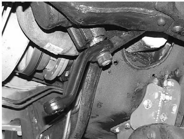
12. Remove the factory steering stabilizer from the frame bracket and save the hardware. Remove the bracket from the frame and discard and save the hardware.
