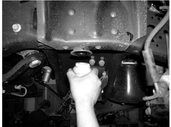
8. Locate the two rivets on the bottom of the coil bucket. Using a die grinder with a cutoff wheel, make an X cut on the face of the rivet. Next, using an air chisel, remove the rivets from the bucket and frame. Using a drill, drill the two holes out to 1/2".
