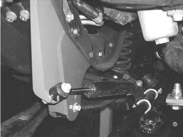
27. Locate the factory alignment cam. Completely remove the pinch bolt on the I-Beam and remove the factory alignment cam and discard. Locate the supplied FT594 alignment cam and place it into the I-Beam where the stock cam was. Re-install and tighten the pinch bolt. SEE PHOTO BELOW.
