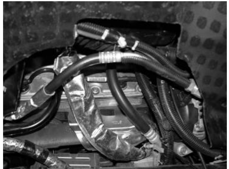
Photo shows bent A/C line
