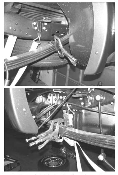
4. Separate the individual leafs and install the provided FT30275 add a leafs with the new center bolt in a pyramid pattern smallest on the bottom graduating to the longest on top. Locate FT30284 Leaf Spring Spacer and place on the bottom of the stack. Clamp the spacer and springs and tighten the center bolt as not to leave a gap between the springs. Cut the thread of the bolt smooth with the nut. The nut should be on the top of the leaf spring pack. SEE DRAWING ON NEXT PAGE
