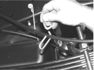
3. Clamp the leaf spring in the middle of the spring and remove the center bolt. (DO NOT REMOVE THE LEAF SPRING FROM THE TRUCK)
