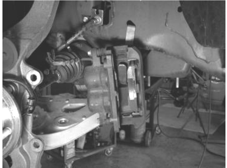
Brake Caliper Shown Hung from Frame
