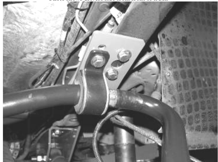
Photo shows sway bar in rear holes for 7.3L diesel from front of truck
