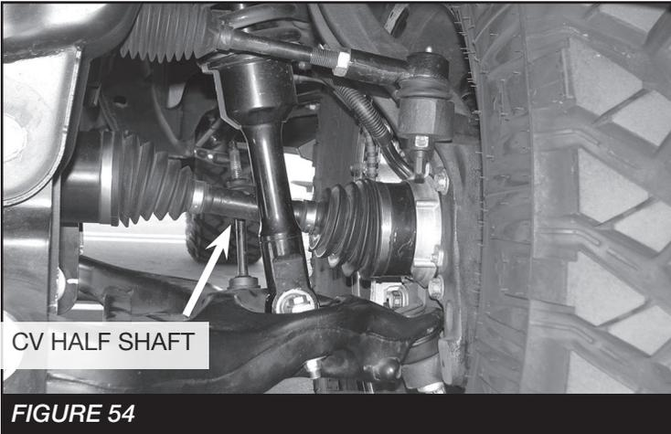
4. If the CV half shaft remains stationary when the wheel/tire is rotated repeat steps 1-3 on the front passenger wheel/tire.
