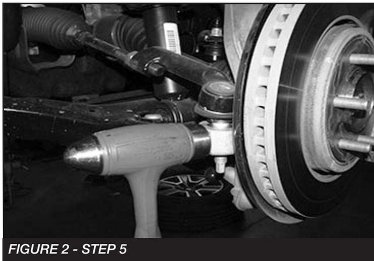
6. Remove the brake caliper and place it next to the frame. Do not overstretch the brake hose when doing so. Retain the hardware for reinstallation. Remove the brake rotor and save. Disconnect the vacuum lines attached to the rear of the hub assembly. Allow the vacuum lines to hang freely. Remove the electronic stability control (ESC) sensor from the top of the hub. Cover the sensor to keep it free from dirt and debris. **SEE FIGURE 3**
