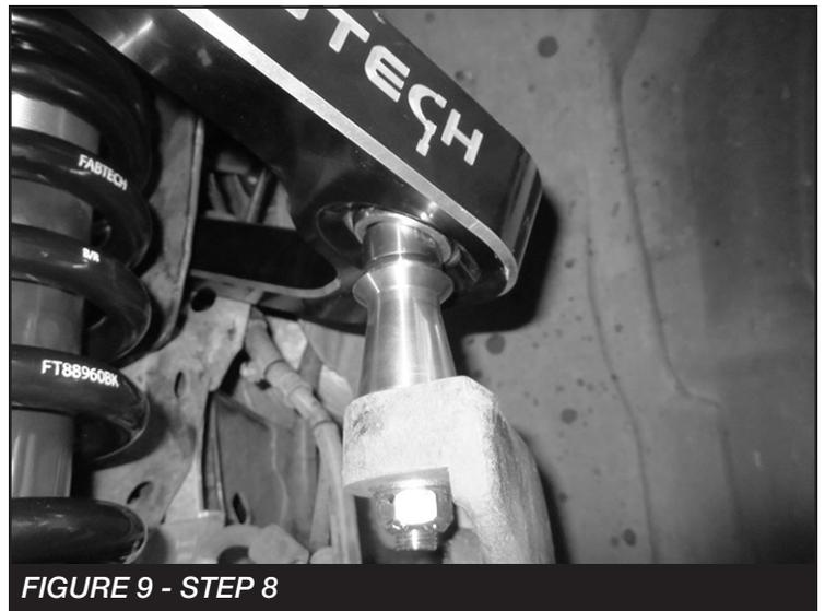
9. Insert the FT30830 (Upper misalignment) onto the top of the bearing assembly. Then, install the supplied 1/2" x 1" bolt. Torque to 120 ft-lbs. **SEE FIGURES 10-11**
