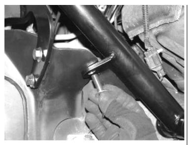
11. Locate the factory bumpstop mounting cup on the frame, use a die grinder and remove the retaining tabs on the inside of the mounting cup. SEE PHOTOS BELOW.
