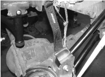
18. Locate FTS23016 Driver Dirt Logic Coilover w/ Resi mount. Install the mis-alignments into the bottom of the coilover. Then install the coilover into the shock mount on the axle mount. Using the factory lower shock bolt, attach the bottom of the coilover to the axle mount. SEE PHOTOS
