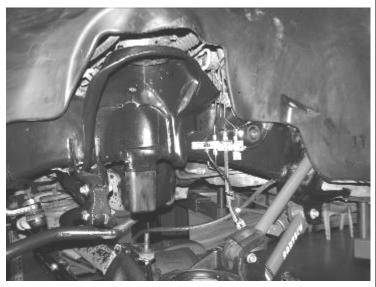
3. Locate the template sections that are included in the back pages of the instructions. Cut the sections out and match them up accordingly, and tape them together. Using masking tape, tape the inside of the coil bucket. Put the template into the bucket so that the bottom of the template is at the bottom of the frame. Use the tape to hold the template to the bucket. Trace the top of the pattern to the coil bucket. SEE PHOTOS IN NEXT COLUMN & PAGE.
