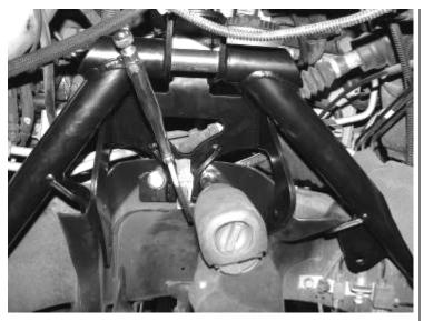
10. With the hoop and support tubes torqued, mark and drill the remaining five 7/16" mounting holes on the tubes to the bucket. Drill the holes to 7/16" and attach with the supplied 7/16" x 1 1/4" bolts & hardware. \*\* Torque to 83 ft. lbs. SEE PHOTOS BELOW & ON NEXT PAGE.
