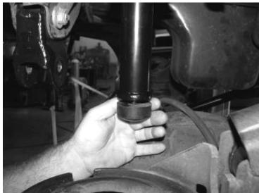
13. Working from the passenger side, locate FT44096BK Pass. Rear Support Tube, FT113 Frame Sleeve, FT44059 Frame Flag, & the supplied 1/2" x 6" bolt w/ hardware. Insert the sleeve into the frame & follow with the support tube with the 6' bolt. Place the flag on the back of the frame followed with the nut and washer. Rotate the flag so it is flat on the frame and the bolt is straight. Leave loose. SEE PHOTO BELOW.
