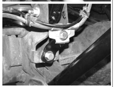
17. Locate FT30192BK Limit Straps and the supplied four 9/16" washers. Remove the factory upper link arm bolt (DO NOT REMOVE THE LINK ARM FROM THE MOUNT) from the link arm at the differential. Put the factory bolt through the limit strap, then 2 of the 9/16" washers, and back through the mount & link arm and install the factory nut. Leave loose at this time. SEE PHOTOS IN NEXT COLUMN.
