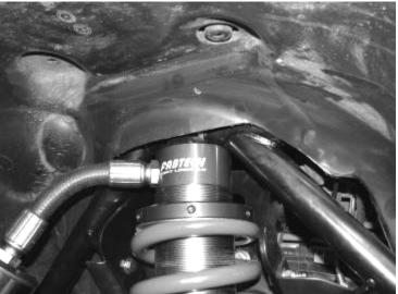
22. Locate the supplied Billet Resi clamp and attach the resi to the front support tube. Mount the resi so that is it as far up and forward as possible. SEE PHOTOS BELOW & ON NEXT PAGE.
