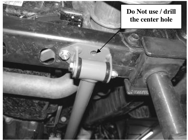
Note position of the Impact Tube Mount.
