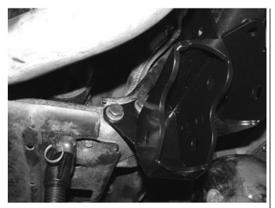
16. Locate and insert the three FT177 frame sleeves into the three holes in the side of the frame. Re-install the pocket using the supplied 1/2" hardware. The rear bolt uses a flat washer on the bolt on both sides of the frame and nut tab FT44154. The front of the pocket gets the 1/2" button head bolt with one flat washer and nut tab FT44152. Torque the 1/2" hardware to \*\*127 ft-lbs and the 14mm hardware to \*\*215 ft-lbs. SEE PHOTOS BELOW.
