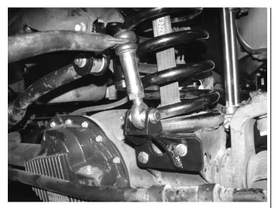
32. Working with both sides, locate FT44137 Brake Line Bracket & the supplied 1/2" x 1-1/4" hardware. Drill the factory mount on the axle and the brake line bracket to 1/2". Attach the Fabtech bracket to the factory mount on the axle with the 1/2" bolts. Attach the brake line bracket to the new Fabtech bracket. Torque to \*\*127 ft-lbs. SEE PHOTOS BELOW.
