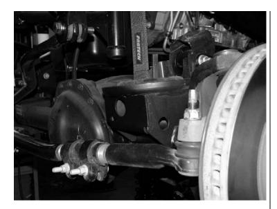
28. Locate FT44155BK Sway Bar Mount, FT44157 Nut Tab, and 7/16" hardware. Attach the new Sway Bar Mount to the lower coil spring mount using the 7/16" hardware and the Nut Tab. Mark the outer hole, remove the new mount, drill out the remaining hole and re-install the mount. On passenger side, measure factory track bar bolt and drill FT44156BK Sway Bar Mount to same diameter as factory bolt. \*\* Torque to 83 ft-lbs. SEE PHOTOS BELOW
