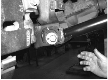
21. Locate the assembled FT44148BK upper link arms. Attach the link arms to the new frame pocket using the supplied 3/4" hardware (DO NOT ATTACH TO AXLE MOUNT AT THIS TIME). The uni-ball goes into the new frame pocket. **Note: When installing the upper links, make sure that the gussets are facing up.** Leave the link arm bolts loose at this time. **If installing dual shock do so before moving on to step 22.** SEE PHOTO BELOW.
