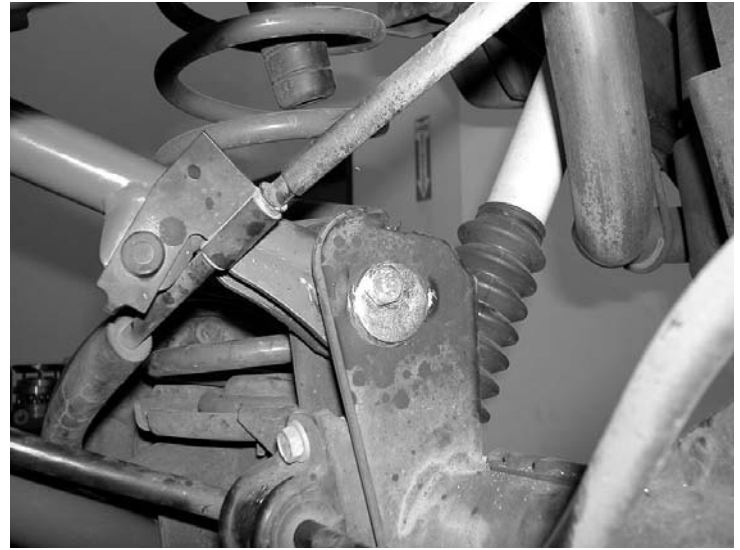
Photo shows cams installed with optional link arm
