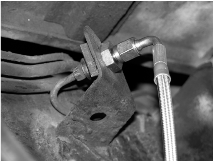
Hose needs run down from factory hard line and parallel the frame
