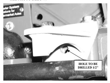
Remove the bracket and drill the hole in the upper axle perch bracket on your mark using a ½ drill bite. SEE PHOTO IN NEXT COLUMN.
