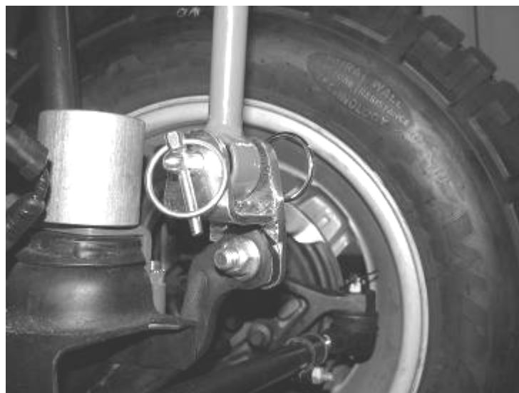
Picture shown with coilover bumpstop spacer
