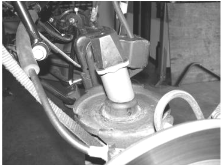
Picture Shown With Bump Stop Installed
