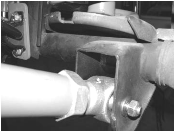
Axle Mount Shown With Grease Fitting Facing Up
