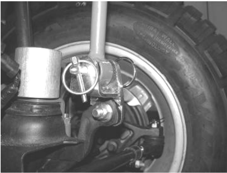
Picture shown with coilover bumpstop spacer
