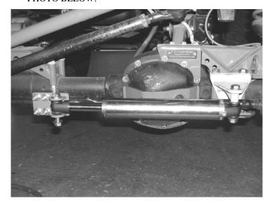
8. Now with the wheels in the straight position set the stabilizer so it has 3 ¼ inches of shaft showing and tighten the U-bolts. Torque to 15 foot lbs. SEE PHOTO BELOW.
