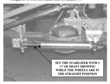
9. Turn the wheel all the way to left then all the way to right to make sure the stabilizer is letting the vehicle turn full left and full right before driving.
