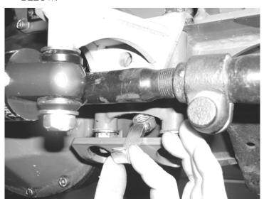
6. Find p/n FT50340 and p/n FTS31UBK U-bolt Kit and install just to the left of the original stabilizer hole in the center link when looking at the vehicle head on. Leave the bracket loose. SEE PHOTO ON NEXT PAGE.
