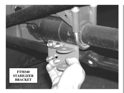
Find p/n FT85005-U steering stabilizer and install in the new brackets with the top cap facing the driver side of the vehicle and the Schrader valve facing away from the center link. Tighten the stabilizer bolts and torque to 55 foot lbs. SEE PHOTO BELOW.
