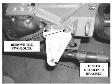
3. Install the bracket leaving the bolts loose. Mark the center of the hole on the vertical part of the bracket to be drilled ½". SEE PHOTO BELOW.
