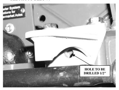
Remove the bracket and drill the hole in the upper axle perch bracket on your mark using a ½ drill bit. SEE PHOTO IN NEXT COLUMN.
