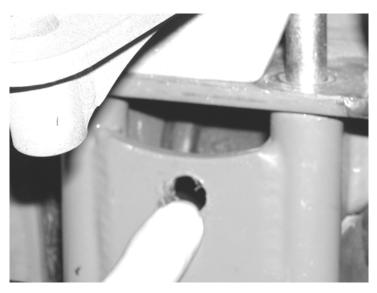
5. Reinstall the stabilizer bracket p/n FT50339 using the ½ bolts that came out of the upper axle perch. Find the nut tab p/n FT50341 and the ½-13x1 ½ bolt supplied and install it in the hole you drilled. Torque bolts to 60 foot lbs. SEE PHOTO BELOW.
