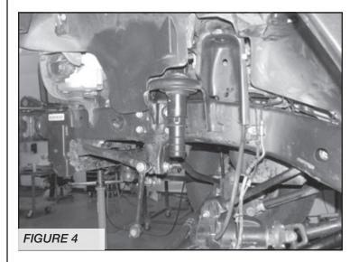
Install the new FT50391BK front coil spring. SEE FIGURE 5
