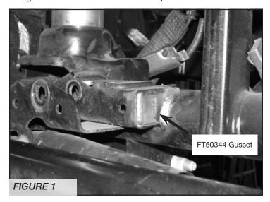
Locate FT50343 gusset, position it onto the top of the axle and trac bar mount. Weld the gusset as shown in the photo. SEE FIGURE 2
