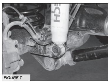
11. Locate FT50261BK Front Sway Bar End links, FT50048 & FT50089 bushing and sleeve kits. Press one bushing and one sleeve from the supplied bushing kit into each end of the end link. With the factory hardware, connect the new end link to the sway bar, then using the supplied ½" x 2-3/4" bolt, nut and washers, connect to the lower sway bar mount. Torque the sway bar hardware to 45 ft-lbs. SEE FIGURE 8
