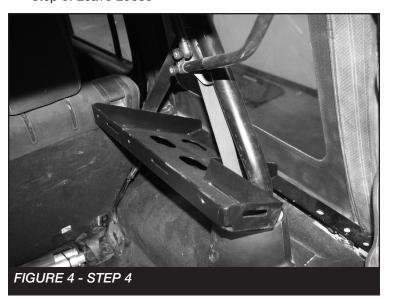
Install FT50660 (Center Tray) using the supplied 3/8" hardware. Torque to 44 ft-lbs. SEE FIGURE 5
