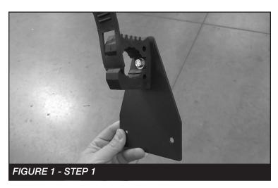
Install the Shovel mount assembly to the inside set of holes on the Fabtech cargo rack using the supplied 1/4" x 3/4" hardware. Torque all hardware to 12 ft-lbs. SEE FIGURES 2-3. Repeat steps for the other mount.
