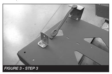
Install the supplied ball stud to the rear bracket using the supplied 5/16" washer and nut. Torque to 25 ft-lbs. SEE FIGURE 4
