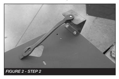
Install FT50820 (Rear bracket) to the set of holes towards the rear of the vehicle using the supplied 5/16" hardware. Torque to 25 ft-lbs. SEE FIGURE 3
