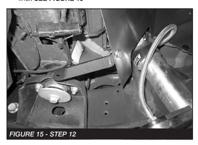
13. Push the liner into the wheel well placing the new bracket against the rear frame support. Mark and drill a 9/32" hole next the factory cut out on the frame support. Then, install the bracket using the supplied 1/4" x 3/4" hex bolt, nut and washers. **SEE FIGURES 16-17**
