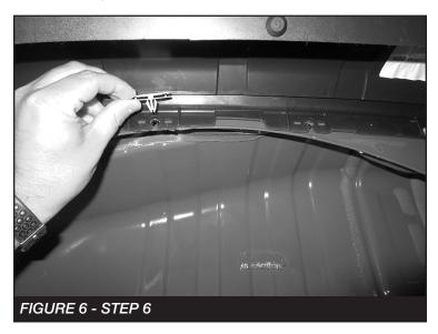
Installation with Fabtech fenders- Counting from the front of the vehicle remove the 1/4" hardware and/or brackets from the 3rd, 4th & 5th inside the fender. SEE FIGURE 7
