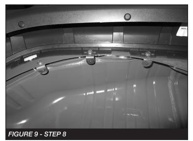
9. Install the Driver side fender liner to the three fender tabs using the supplied 1/4" x 3/4" Buttonhead bolts and washers. Leave loose. NOTE: The liner will need to be installed so it sits inside of the wheel well pinch weld. Install three FT90173 (Push in rivets) into the inner liner and factory holes on the vehicle. SEE FIGURE 10
