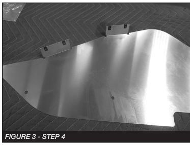
Install FT50870 (Driver Top Liner) to FT50871 (Driver Side Liner) using the supplied 8-32 buttonhead bolts and washers. SEE FIGURES 4-5 Repeat for the passenger side.
