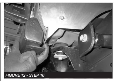
11. Push the liner into the fender well and place the new bracket against the factory pinch weld. Mark the hole for drilling. Use a 9/32" drill bit to drill the hole. Install the bracket using the supplied 1/4" x 3/4" hex bolt, washers and FT50905 (Nut Tab). **NOTE: If installing on a vehicle with factory installed rock sliders the bolt will have to be installed from the backside. SEE FIGURES 13-14**
