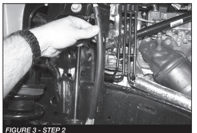
3. Ubolt and remove both driver and passenger side brake line brackets from the axle spring perch. **SEE FIGURE 4**
