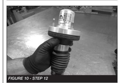
On the factory lower coil spring perch. Remove the plastic coil isolator. Use a drill with a 1/2" drill bit and drill out the existing factory hole on both driver & passenger sides.
