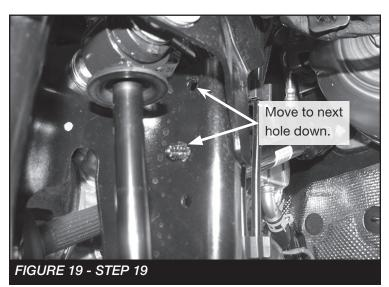
19. Reinstall the diff breather hose by moving the metal clip up the hose 2" **SEE FIGURE 18** and the christmas tree fastener into the next hole down. **SEE FIGURE 19.**
