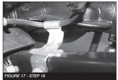
link arm brake line bracket upward an inch to give the line some relief at full extension. SEE FIGURE 17
