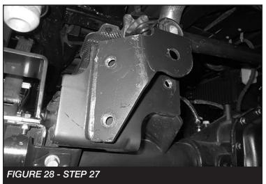
27. Install the FT50783 (Rear track bar bracket) onto the factory bracket. Insert the supplied 9/16" X 3" bolt. Mark the 3 holes using the new bracket as a template. SEE FIGURES 26-28. Remove and drill the 3 holes using a 7/16" drill bit.
