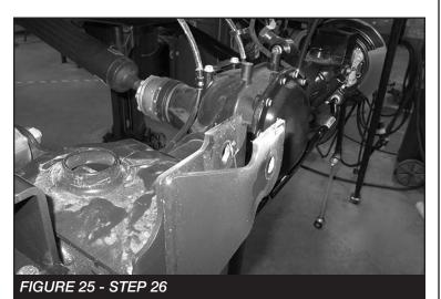
26. Locate the factory rear track bar bracket. Mark a straight line on the front and back before the 90 degree bend. Remove the track bar from the axle bracket and cut the
