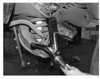
3. Take the driver's side spindle, marked FT2588-7D, and install it onto the upper and lower ball joints. Reinstall the original castle nuts and torque to factory specs. Install a supplied cotter pin in each castle nut, **DO NOT REUSE THE ORIGINAL COTTER PINS.**
