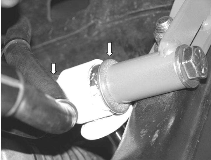
arrows show large USS flat washers on both sides of shock
