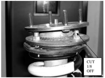
8. Install coilover on the truck starting at the top. Torque nuts to 30 ft.lbs. SEE PHOTO BELOW.
