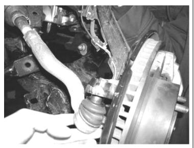
4. Remove the bottom coilover bolt and save. Remove the four nuts attaching the coilver to the coilover mount, save hardware. Remove the coilover from vehicle. SEE PHOTO BELOW.
