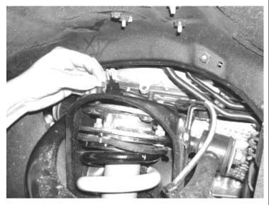
9. Using a long punch twist the lower shock eyelet so it will line up with the shock mount on the lower arm. Install the lower end of the shock reusing the factory bolt and torque to 120 ft. lbs. SEE PHOTO IN NEXT COULUMN.
