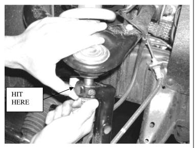
3. Loosen the tie rod nut. Using the appropriate tool to remove the tie rod end. Save all hardware (Use care not to damage threads.) Disconnect the factory swaybar endlinks and save with the hardware. SEE PHOTO BELOW.
