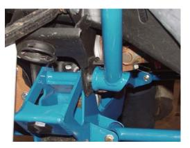
5. Place the front leg of the hoop over the removed steering box bolt hole and reinstall the stock steering box bolt, nut and washer. Leave loose.
