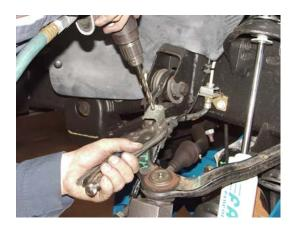
9. Locate the lower shock mount and place over the factory upper control arm. Using 3/8" x 2" cross bolts, nuts and washers attach arm with the brake hose retaining clamp to the inside of the control arm. Note must use 3/8" x 2" bolts on the mount eyes closest to frame to allow for shock clearance. Use 3/8" x 2-3/4" bolts, nuts and washers for the mount holes to the outside of the vehicle under the control arm. Leave all bolts loose. SEE BELOW PHOTOS
