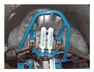
13. Repeat same procedure for passenger side. Except step two, remove the factory differential mounting bolt on the side of the frame rather than the steering box bolt. For ease of installation cut 5/8" off the end of the rear differential mounting bolt that protrudes through the frame. Follow all other steps the same as the driverside.
