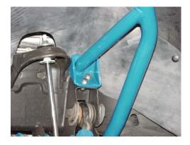
7. Tighten the steering box bolt to 90LBS and the lower control arm rear bolt to 90LBS
