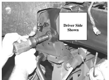
12. Locate and remove the nut and washer that retains the stock lower control arm pivot bolt towards the rear of the vehicle. Do not remove the bolt, only the nut and washer.
