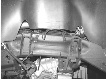
11. Working from the driver side of the vehicle, locate and remove the steering box bolt on the outside of the frame rail closest to the upper control arm. SEE PHOTO BELOW.
