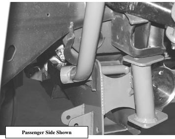
14. Place the front leg of the hoop over the steering box bolt hole and re-install the stock steering box bolt, nut, and washer. Torque the steering box bolt to 110lbs and the rear lower control arm bolt to 90 lbs. SEE PHOTO BELOW
