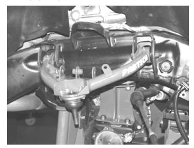
6. Attach the steering knuckle to the upper control arm using the provided ½" SAE Flat Washer over the new ball joint
