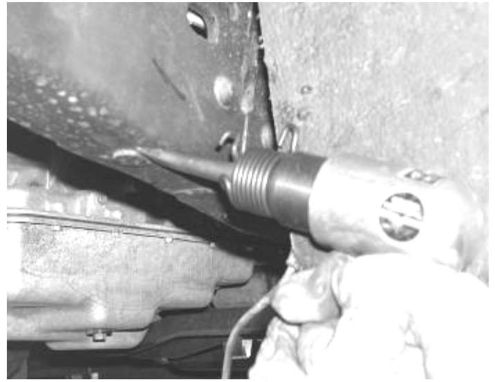
Removal of rivet with an air hammer
