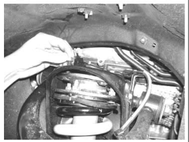
9. Using a long punch twist the lower shock eyelet so it will line up with the shock mount on the lower arm. Install the lower end of the shock reusing the factory bolt and torque to 120 ft. lbs. SEE PHOTO IN NEXT COULUMN.
