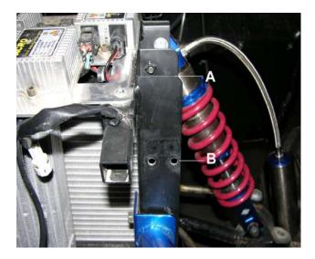
With the use of a 5/16" drill bit, drill out the 2 holes for the Resi mount. Locate hardware bushing kit # FT86013. With the Resi mount on the inside of the core support and 2 5/16-1 bolts, 4 5/16 washers and 2 5/16 nuts begin to bolt on the Resi mount to the Rhino. Once the Resi mount is in position locate the 2 hose clamps and attach the reservoir to the Resi mount and tighten the hose clamps.
