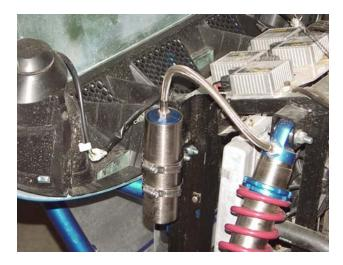
Once you have completed the driver side move and repeat the steps on passenger side. Once both sides are completed and the reservoirs are mounted with the Resi mounts, reinstall the front wheels and torque the wheel nuts to specs. You have now completed the front shock installation.
