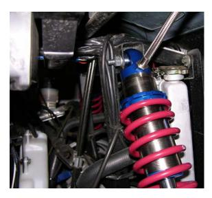
Locate the Dirt Logic shock FTR60130 and with the reservoir hose facing the installer mount the top cap first and the rod end second.
