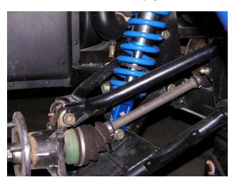
"C" channel support beam in the rear of the Rhino. Measure from point A to B 2 1/4" (See Picture) and mark a horizontal line with a marking pen. Locate Resi mount #FT83178 which has an angle and line it up along the
