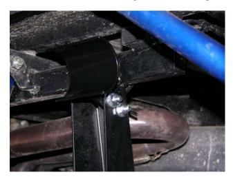
Once you have completed the driver side move and repeat the steps on passenger side. Once both sides are completed and the reservoirs are mounted with the Resi mounts, reinstall the rear wheels and torque the wheel nuts to specs. You have now completed the rear shock installation.
