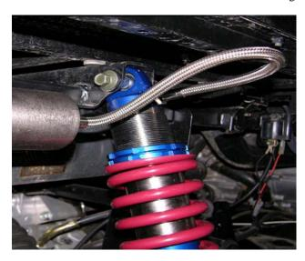
on the driver side of the Rhino, remove the bolt and nut from lower stock shock. Now remove the bolt and nut from the upper shock mount, and with caution remove the shock from the Rhino. Locate the Dirt Logic shock FTR60133 and with the reservoir hose facing the installer mount the top cap first and the rod end second. Tighten the stock bolts and nuts to the factory specs. Locate the
