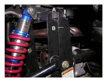
With the Resi mount on the inside of the core support and 2 5/16-1 bolts, 4 5/16 washers and 2 5/16 nuts begin to bolt on the Resi mount to the Rhino. Once the Resi mount is in position locate the 2 hose clamps and attach the reservoir to the Resi mount and tighten the hose clamps.
