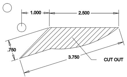
Cut out this pattern for use on both sides of the truck.
