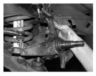
7. Grind the heads off the rivets securing the steering stop to the backside of the LCA. Using a punch or air chisel, remove the rivets and steering stop from the LCA. SEE PHOTO BELOW.
