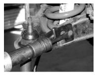
8. Take the supplied cutting pattern and mark the lower control arm. SEE PHOTO BELOW AND DIAGRAM AT END OF INSTRUCTION SHEET.
