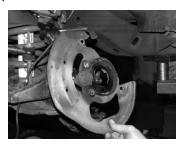
4. Grind off the rivet securing the ABS wire clamp to the dust shield and remove the clamp. Mark the top corner of the dust shield, as shown, and trim the marked area with sheet metal shears. SEE PHOTOS BELOW.
