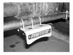
4. Locate both the supplied FTS7001 or FTS6601 stabilizers, attach one FT140357 shock stud to each end of the stabilizer, attach the stabilizer to the mounting brackets, mounting the body of the stabilizer on the out board side. Torque shock stud bolts to 65 ft lbs. SEE PHOTO BELOW.
