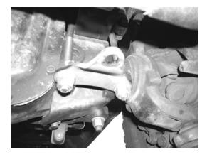
3. Locate the supplied FT8008-1 center bracket, using the supplied u-bolts attach the bracket to the center link. The bracket will need to be centered on the center link, this can be done by measuring from each tire to the center u-bolt. Torque to 15 ft lbs. SEE PHOTO BELOW.
