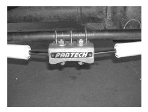
5. Cycle steering left to right and check for adequate clearance on the stabilizers. If either stabilizer bottoms out you will need to adjust the center bracket to allow for proper clearance.
