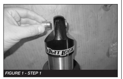
Install FT20980 (Upper mount) into the coilover using the supplied 1/2" hardware. Torque to 106 ft-lbs. SEE FIGURE 2
