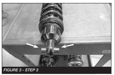
4. Install the coilover using the supplied 7/16" hardware for the upper location and the factory for the lower. Torque the upper hardware to 42 ft-lbs and the lower to 110 ftlbs. **SEE FIGURE 4**
