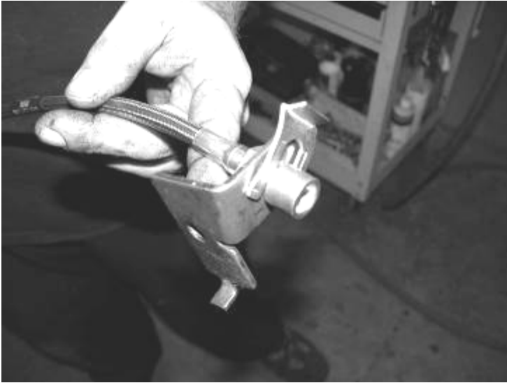
Photo shows brake lines on truck equipped with a Fabtech Long Travel Kit
