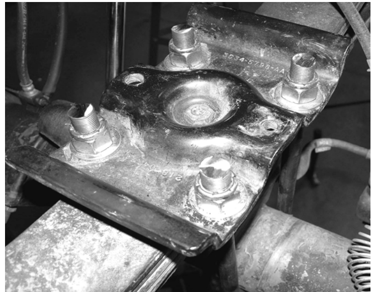
Photo shows Rear hole drilled to 1/2" for new Limit Strap
