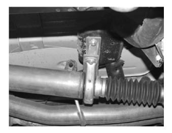
3. After driving the vehicle, re-torque the 7/16" hardware. Because of the added leverage induced by larger tires and lift systems, all driveline vibrations sometimes cannot be completely eliminated.
